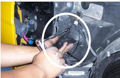
You will have to reposition the filter on the passenger's side as showed on the picture.
