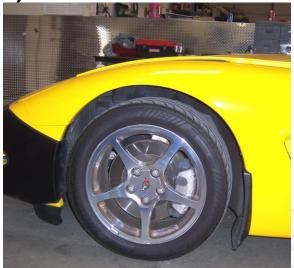
Remove (7) 7mm from the wheel well. Note: Your vehicle may have different size bolts or type of fasteners.
