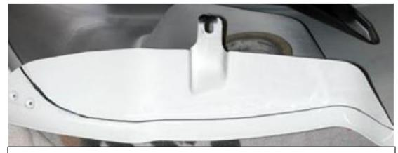
Use a power cutter and grinder to cut and take any sharp edges off. Use black door trip to give it a finish look.
